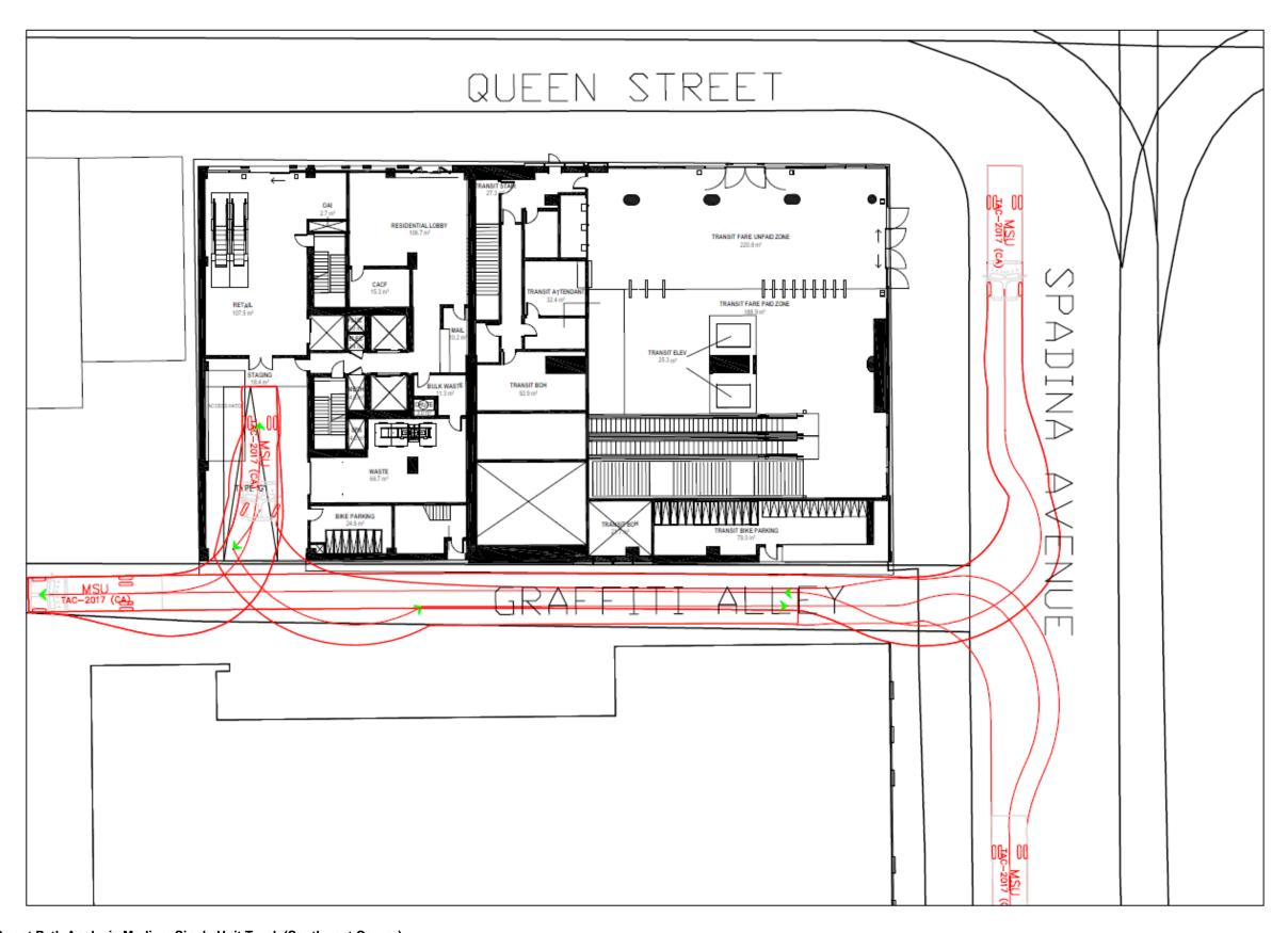
Figure 13: Loading Swept Path Analysis Medium Single Unit Truck (Southwest Corner)
