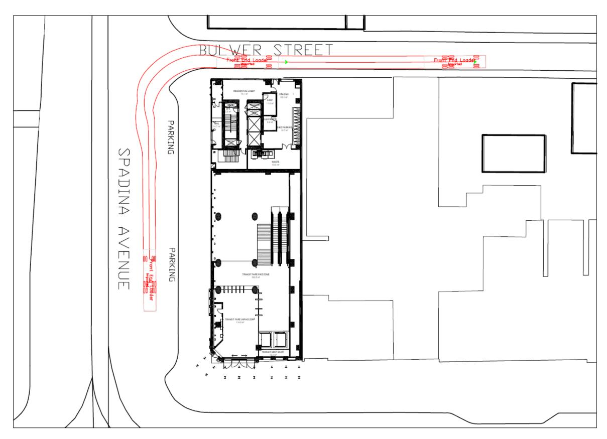
Figure 16: Refuse Swept Path Analysis Front End Loader Refuse Truck (Northeast Corner)
