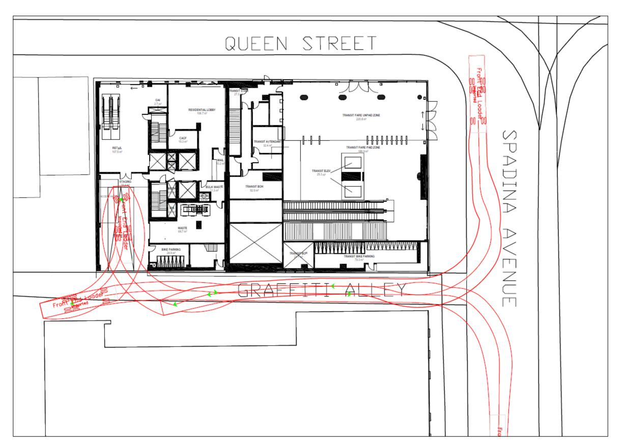
Figure 14: Refuse Swept Path Analysis Front End Loader Refuse Truck (Southwest Corner)
