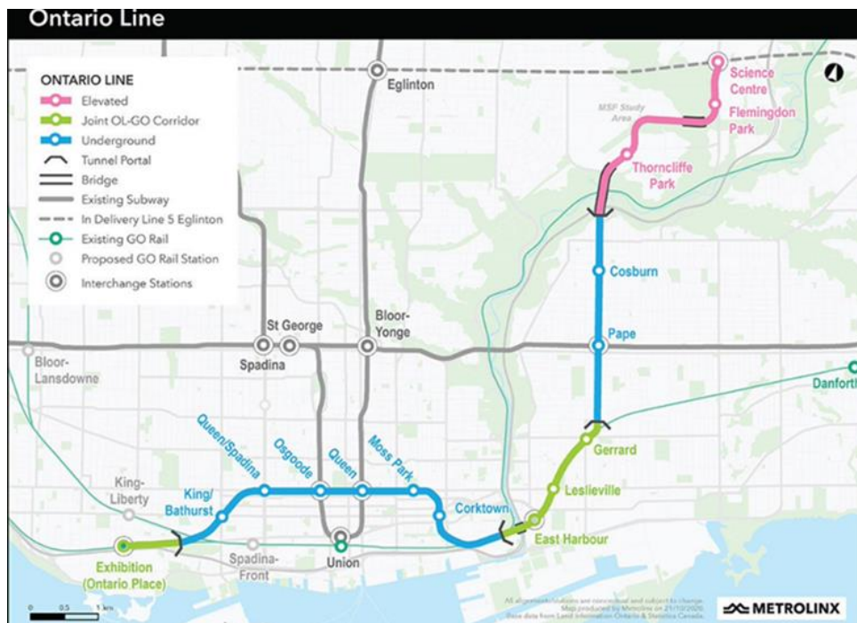
Figure 1-1. Ontario Line Segments
